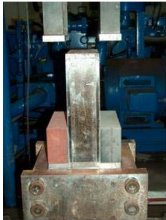
Figure 4 – Modified Die with Bottom Ram Ejecting Brixx
