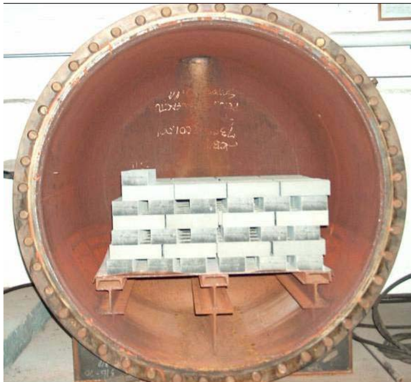
Figure 5 – Brixx in Autoclave after Curing Cycle
