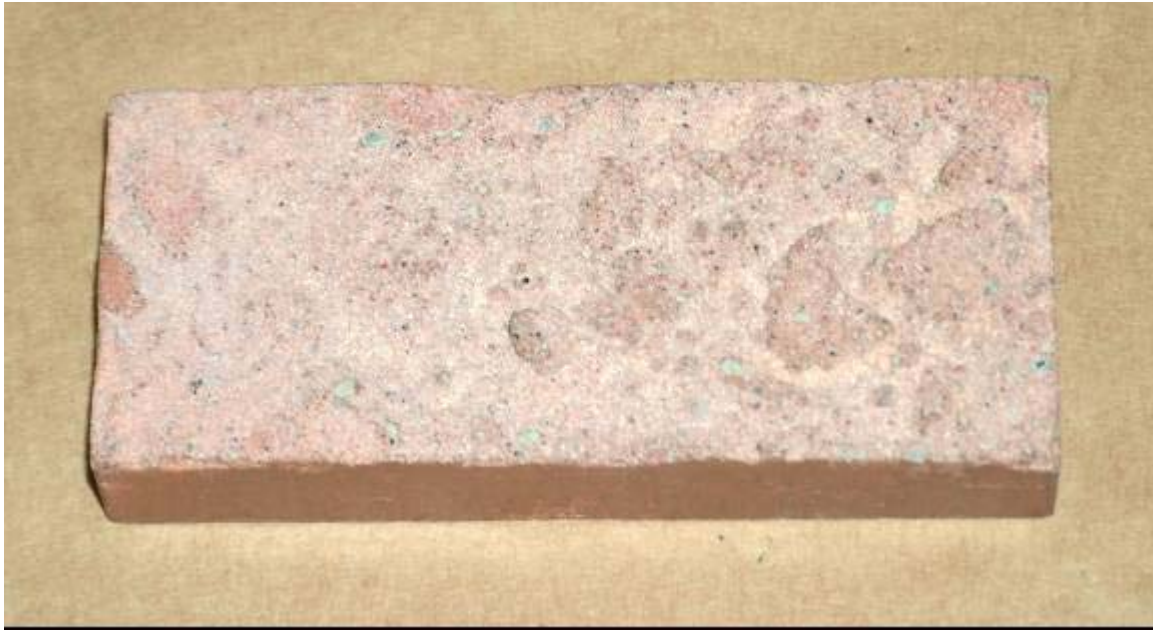
Figure 7 – Laboratory Scale Brixx Produced with Roughened Surface
